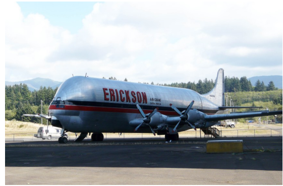
The Mini-Guppy, used for transporting large booster rocket engines in the 1960's
