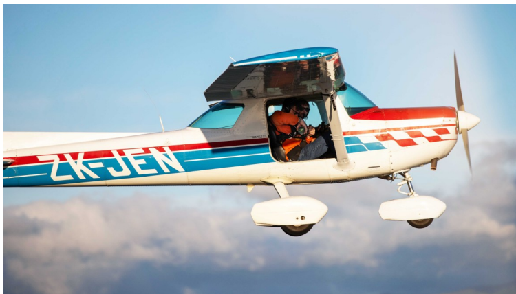
Cessna 152 ZK-JEN set up as Air to Air photography platform (door off).
